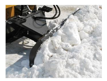
The **114 Series Snow Blade** is available in either hydraulic or manual angle. For Skid Steers, Compact Tool Carriers, and Compact Utility Loaders.
