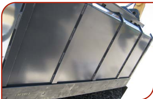
5 wear plates on underside of hopper bin
